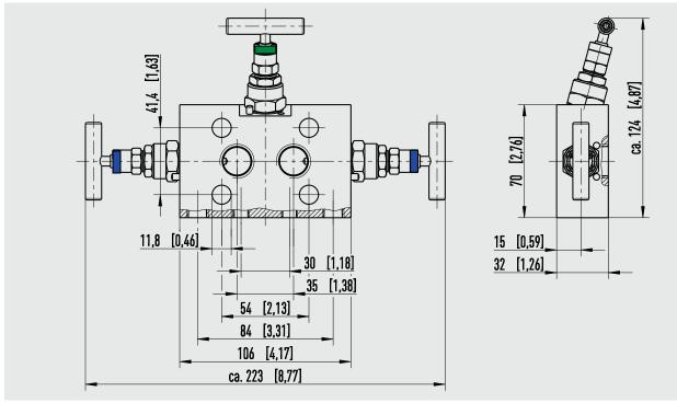
For differential pressure measuring instruments with process connection per IEC 61518 form A or form B Form B: E.g. for differential pressure gauges, WIKA model 732.14, with process connection per IEC 61518 Form A: E.g. for transmitters, WIKA model DPT-10
