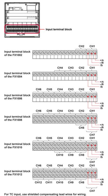
For RTD input, lead wire resistance per wire of 10  $\Omega$  or less. Make the resistances of the three wires equal.
