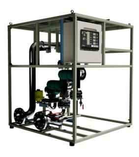
The Rotamass RCx38 are positioned on the main metering lines. There can be 1 to 10 metering lines, depending on the flow range to be measured. These Rotamass therefore measure the general flow and the density of the mixture. By using the density of the three-phase mixture with the densities of the known liquid and gas phase, we then obtain the GVF, or the % of the gas phase in the fluid, at flow conditions P and T.
