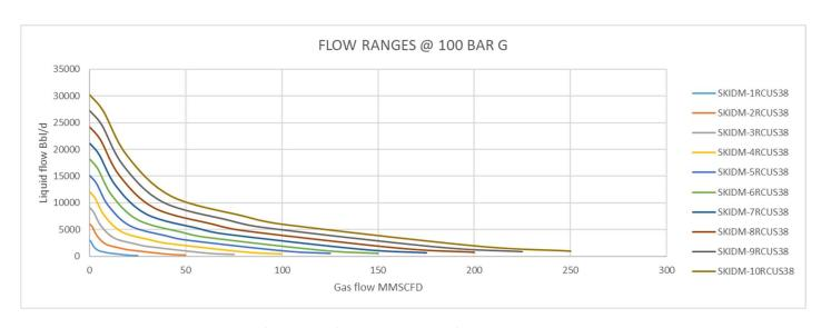
Example of SKIDM performance based on following process conditions: Water density: 1100 kg/m3 / Oil density: 850 kg/m3 / Gas density: 0.8 kg/Sm3 / BSW: 50% / Pressure: 100 barg / Temperature:  $40^{\circ}$ C
