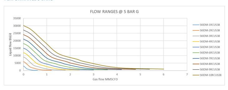
Example of SKIDM performance based on following process conditions:
