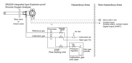
\*1 Shield cable: Use shielded signal cables, and connect the shields to the FG terminal of the converter.
