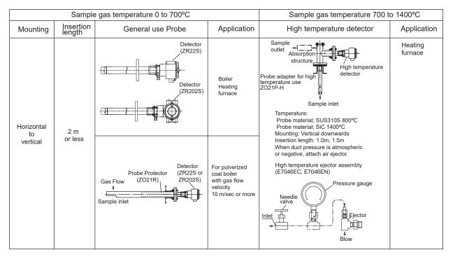
more and up to 0 to 100 vol% O<sub>2</sub> range Linearity: (Excluding standard gas tolerance and the case where the reference gas is by natural convection) (Use oxygen of known concentration (with in the measuring range) as the zero and span calibration gases.) ± 1% F.S.; 0 to 5 or more and less than 0 to 25 vol% O<sub>2</sub> range and sample gas pressure within ± 4.9 kPa
