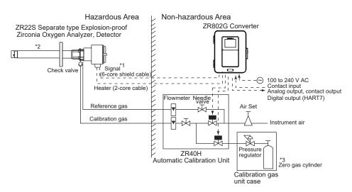
\*1 Shield cable: Use shielded signal cables, and connect the shields to the FG terminal of the converter.
