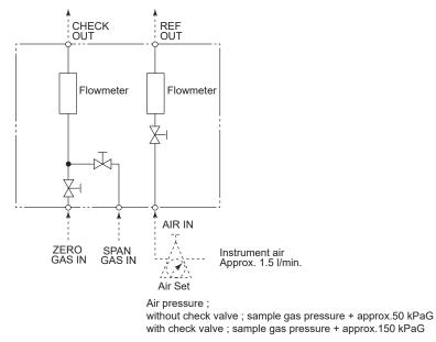
8. Stop Valve for Calibration gas line (L9852CB /G7016XH)
