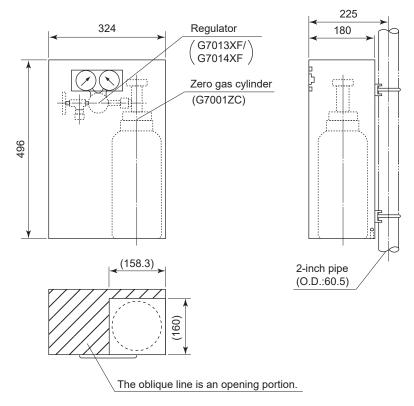
Note: The zero gas cylinder and the regulator valve are not included in the E7044KF
