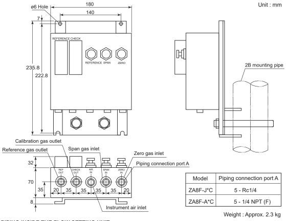
PIPING INSIDE THE FLOW SETTING UNIT
