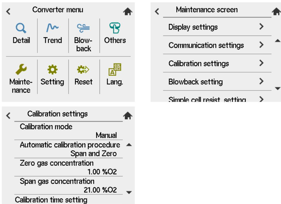
Figure 6.14 Calibration Setup Display
