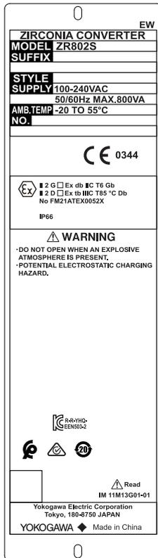
Figure App1.2 Example of nameplate (Design and texts may be changed)
