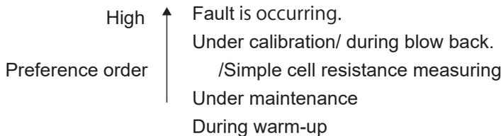
For example, if the output current is set to 4 mA during maintenance, and no output-hold output for during calibration is preset, the output is held at 4 mA during the maintenance display. However, the output hold is released at the time of starting the calibration, and the output will be again held at 4 mA after completing the calibration and when the hold (output stabilization) time elapses.
