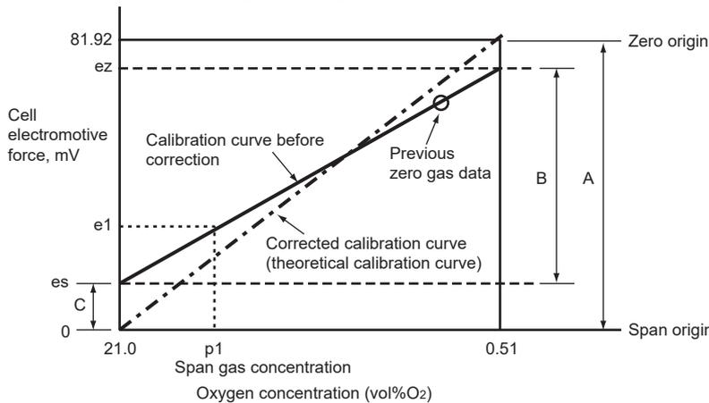
Zero point correction ratio =  $(B/A) \times 100 (\%)$  Correctable range:  $100 \pm 30\%$
