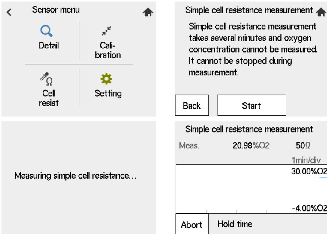
Figure 9.22 Procedure for Simple Cell Resistance Measurement
