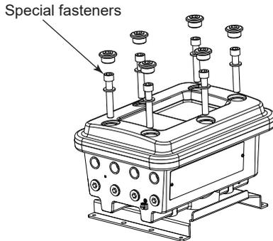
Figure App1.1 Special fasteners
