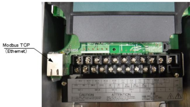
**Figure 4.18** Ethernet connector position
