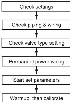
Figure 6.1 Startup Procedure
