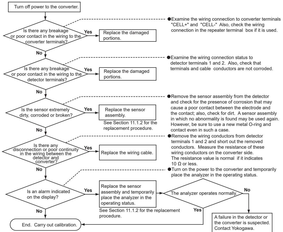
(2) Alarm 017: Heater Temperature Failure
