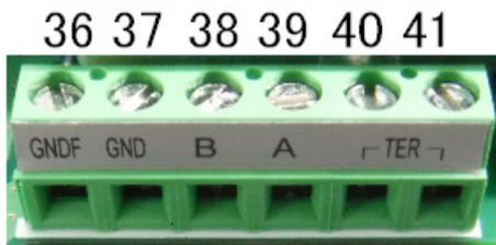
Figure 4.16 RS-485 terminal screw
