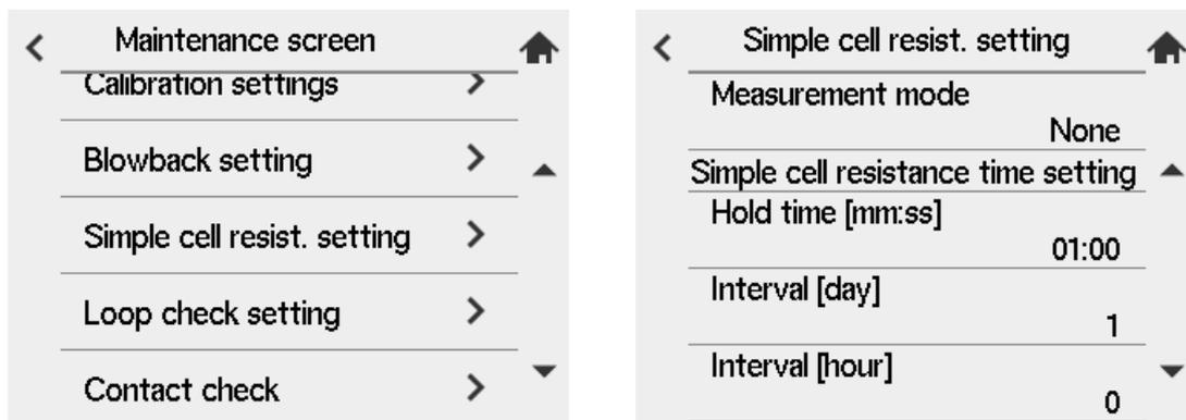
**Figure 9.21 Simple cell resistance setting**
