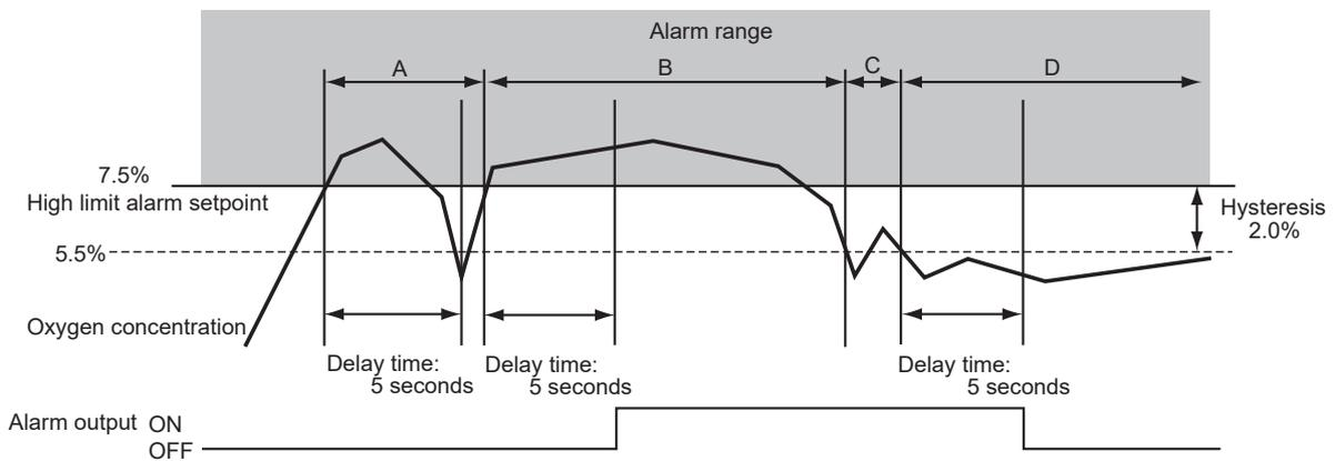
**Figure 7.5 Alarm Output Action**
