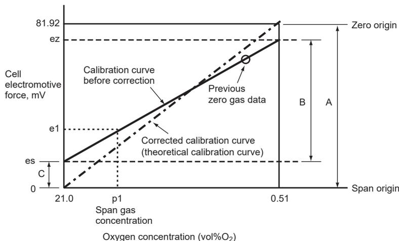
Zero gas correction ratio =  $(B/A) \times 100$  (%) Correctable range:  $100 \pm 30\%$
