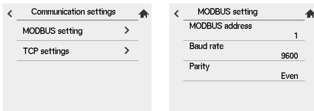
Figure 9.23 MODBUS Communication setup
