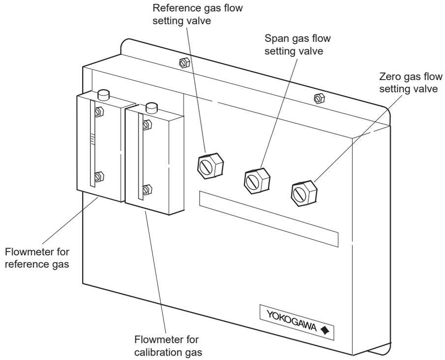
Figure 5.9 ZA8F Flow Setting Unit
