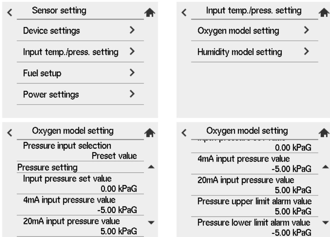
Figure 7.15 Setting Measurement Gas Pressure
