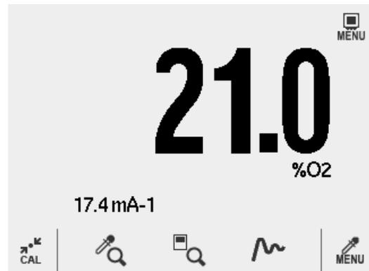
Figure 6.3 Measurement Mode Display
