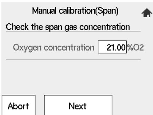
Figure 6.16 Span gas concentration check
