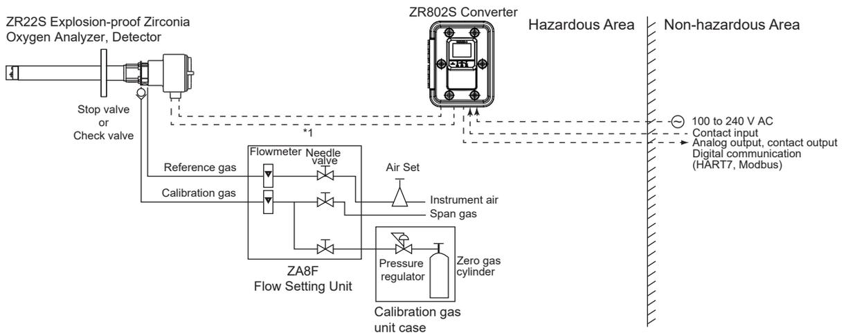
\*1 Shield cable: Use shielded signal cables, and connect the shields to the FG terminal of the converter.
