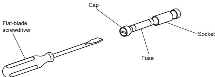
**Figure 10.2** Removing the Fuse
