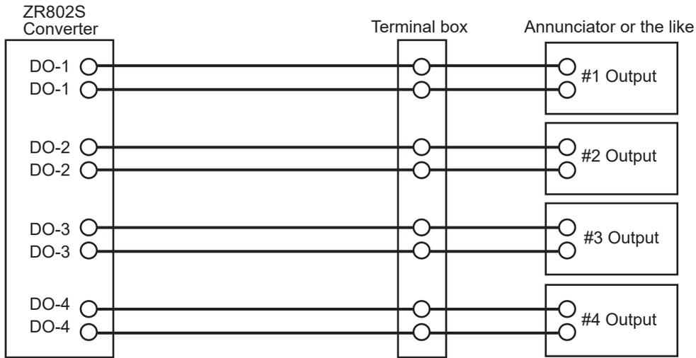
Figure 4.13 Contact output wiring
