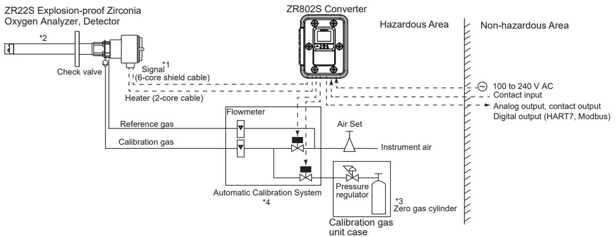
Figure 1.1 System configuration Ex. 1
