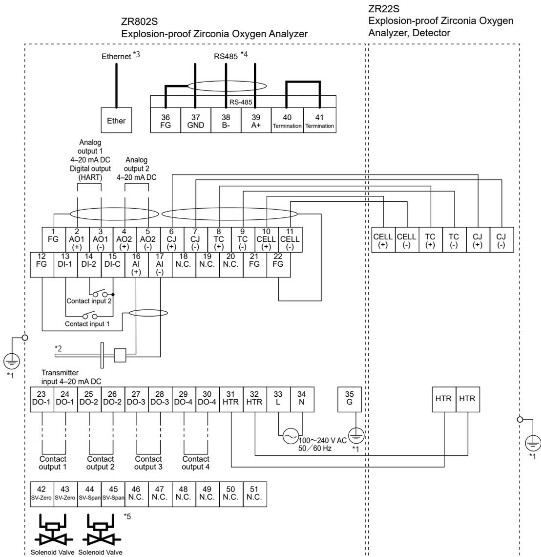
\*1: The ground wiring of the converter should be connected to either the protective ground terminal in the equipment or the ground terminal of the converter case.
