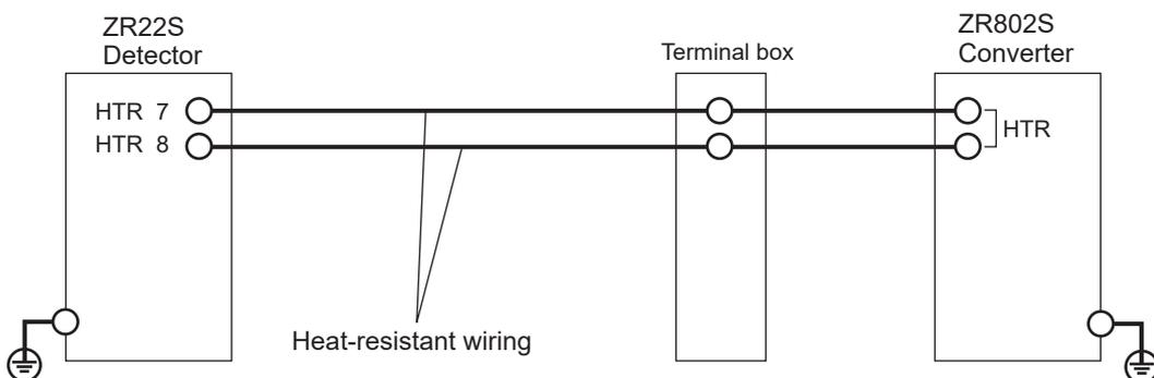
Figure 4.9 Wiring for power to detector heater
