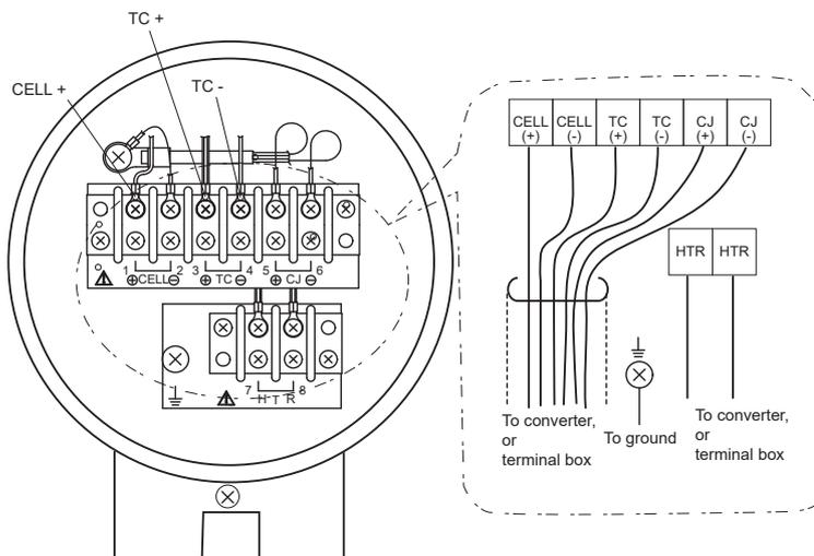
Figure 4.6 Terminal assignment of detector
