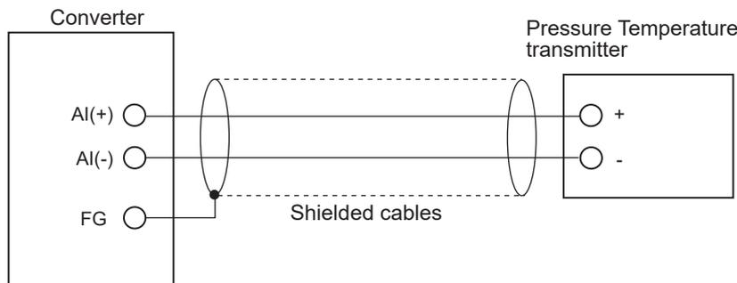
**Figure 4.15 Pressure input wiring**
