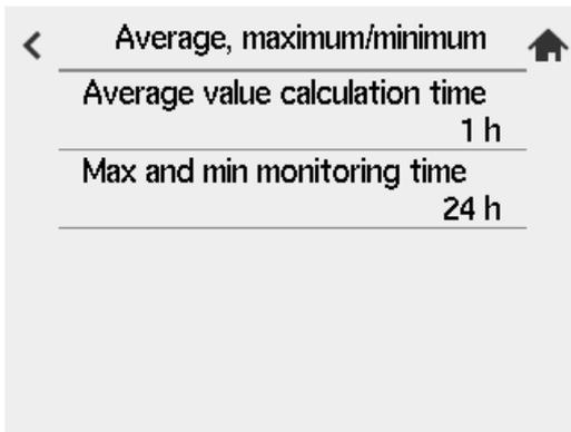
Figure 7.11 Setting the monitoring time of average/max.min. value
