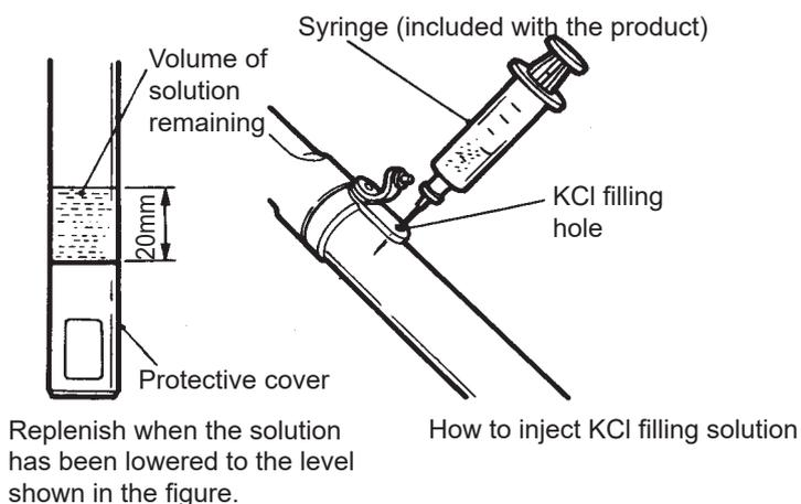
Figure 7.4 How to replenish the KCl filling solution
