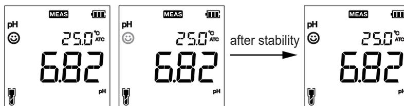
Figure 3.3 Example of pH measurement (auto stability mode)
